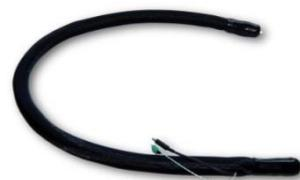
The heated gas line is equipped with plugs to connect to the humidifier for power and thermocouple feedback. The surface temperature is about 40°C, and the maximum inside temperature is limited to 150°C. Higher temperatures are possible on request.
