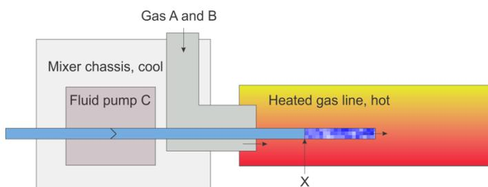
The fluid (component C) is injected to the heated gas through 1/16 inch stainless steel tube. This tiny tube enters the heated gas line tube and the two tubes overlap in the hot zone. When adding large amounts of fluid, the fluid flows into the heated gas line and evaporates there.
