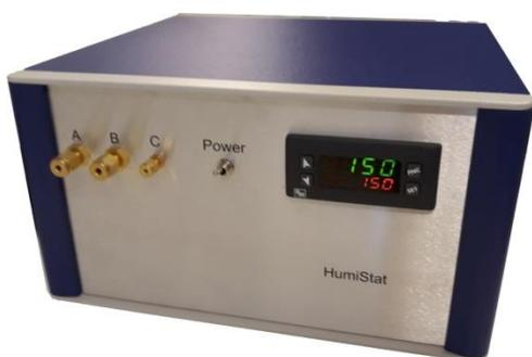
On the front panel are inputs for gases A and B, and input for liquid C, and a PID controller for the heated gas line.
